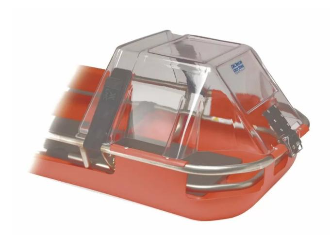
Trusted and proven from years in the field, our Litter Shield attaches to a mount on the litter rail that allows the shield to quickly pivot and nest inside the litter for transporting and storing. A quick-release pin allows the shield to be completely removed when necessary. This lower-profile version makes storage easier, but does not provide as much clearance for the patient's face as the Litter Shield Plus, see below. Each Litter Shield requires a railing clamp.
