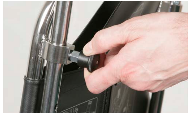
Figure 25 - Chair height adjustment index pin
