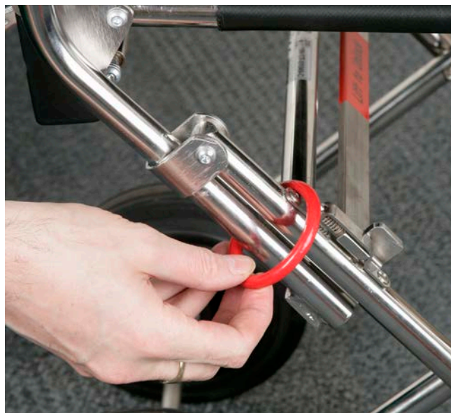
Figure 6 - Securing the chair by deploying safety rings
