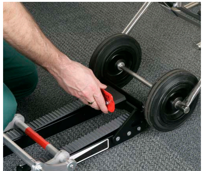
Figure 23 - Releasing the Track from the Chair
