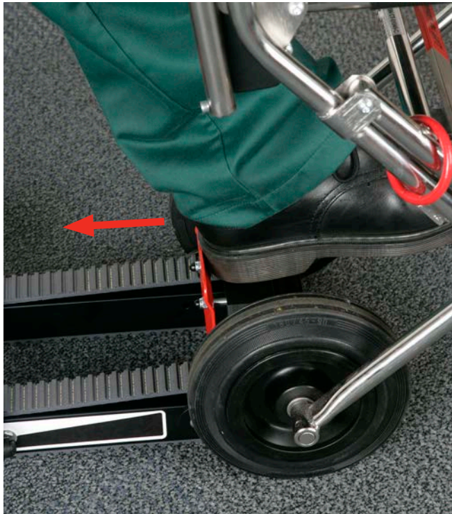
Figure 24 - Removing the Track from an unoccupied Chair
