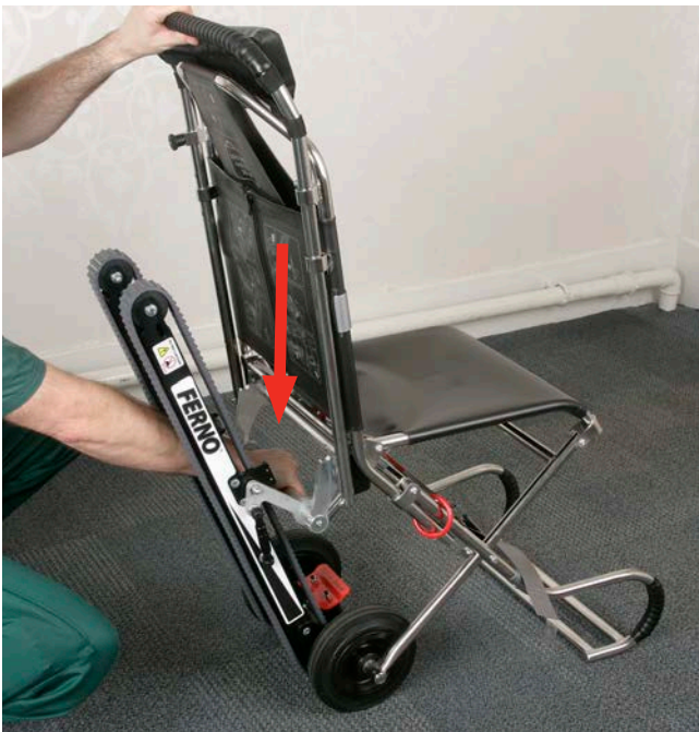
Figure 20 - Using 'Push to Close' bar to stow Track
