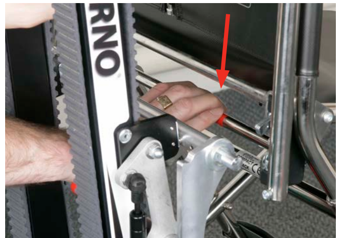
Figure 22 - Releasing Track from push-to-close latches
